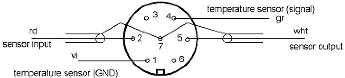
**Built-in socket „Sensor“ at the case:**
